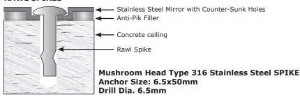
**Installation:** Drill a hole into the base material to a depth of at least 60mm. The tolerances of the drill bit used should meet the requirements of ISO/DIN Standard 8035. Blow the hole clean of dust and other material. Drive the Spike through the appropriate mirror face hole (and frame when used) ensuring the head is sitting firmly against the mirror or frame and recessed as shown in the above diagram.
