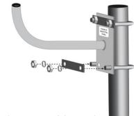
U-Bolt threads through ONE SIDE of the J-Backet
