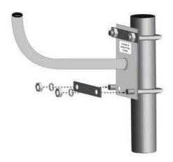
NOTE: U-Bolts thread through ONE side of mounting holes in J-bracket.
