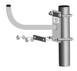
NOTE: U-Bolts do NOT thread through J-bracket mounting holes.
